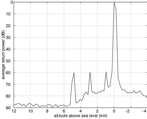
Figure 8: Hardware description language simulation of the spaceborne Data Processor FPGA for the case where weak rain scatterers are observed over the ocean.
