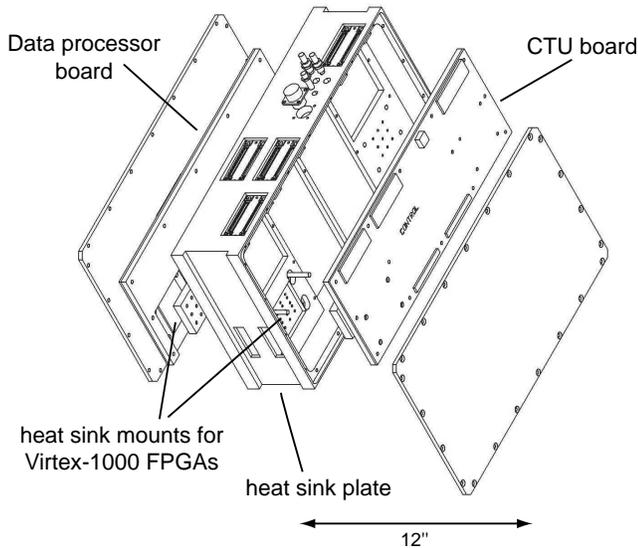
Figure 10: Mechanical chassis design for the spaceborne PR-2 processor/controller.
