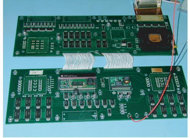
Figure 9: Mounted printed circuit boards for the CTU and bus controller (top) and for the Data Processor FPGAs (bottom).
