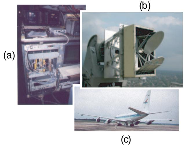
Figure 2: The PR-2 airborne prototype radar: (a) electronic processing and control console, (b) dual-frequency (13 and 36 GHz) antenna feed structure with mechanically scanning reflector, (c) NASA Dryden DC-8 aircraft used for deployment in the 4th Convection and Moisture Experiment (CAMEX-4).
