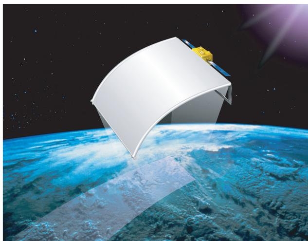
Figure 1: Conceptual drawing of the spaceborne Second-Generation Precipitation Radar (PR-2), with an innovative  $5.3 \times 5.3$  m reflector antenna based upon inflatable/rigidizable technology.
