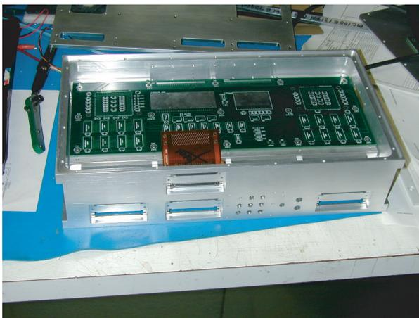
Figure 11: Photo of boards assembled in the aluminum chassis.
