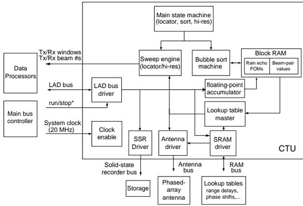
Figure 5: Verilog module design and chip-to-chip interface for the Control and Timing Unit (CTU) FPGA.
