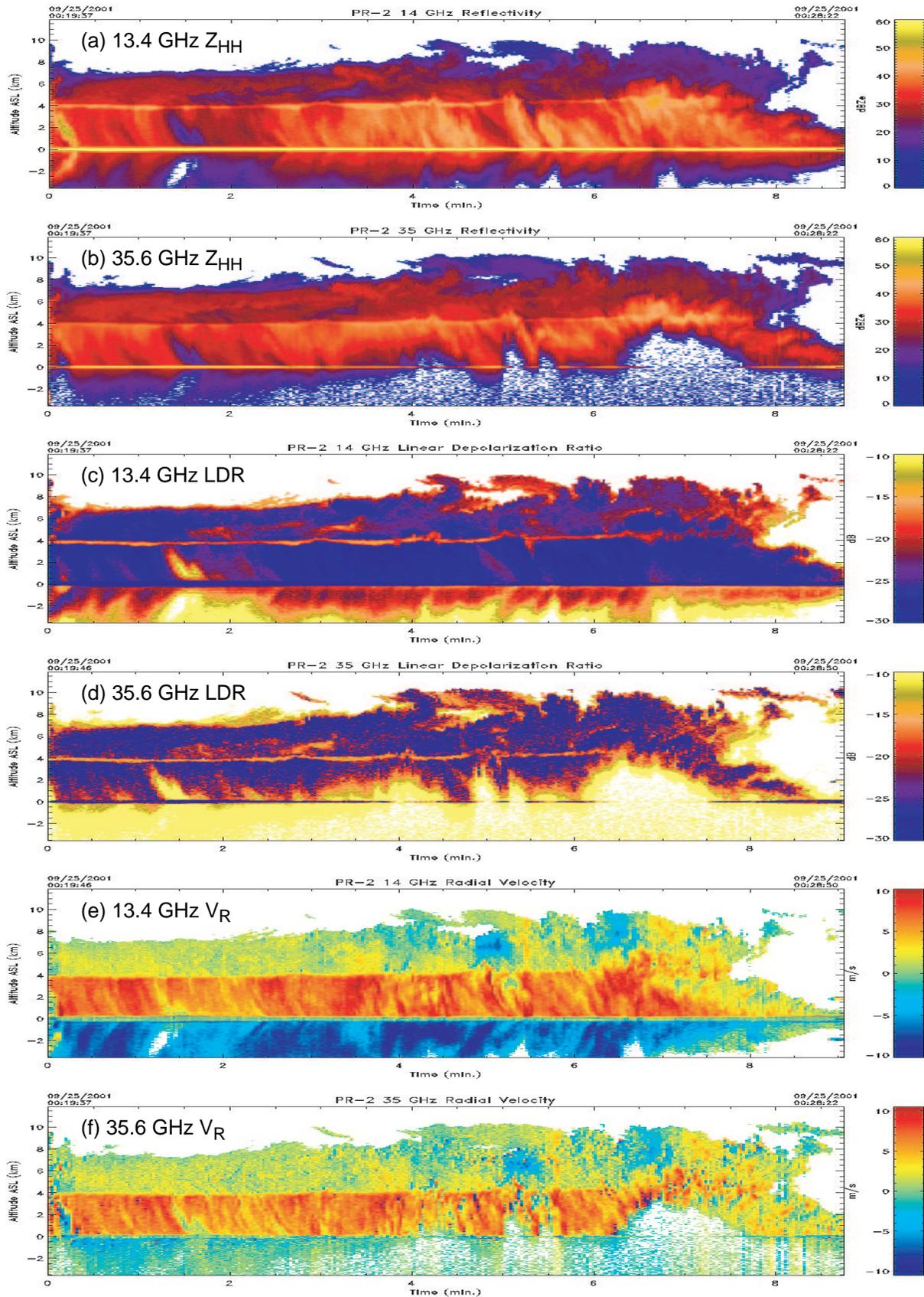
Figure 3: Multi-parameter, dual-frequency (Ku and Ka-band) rainfall data from Hurricane Humberto, taken with the PR-2 Data Processor during CAMEX-4: (a)–(b) H-pol rain reflectivity data. (c)–(d) Linear depolarization ratios. (e)–(f) Vertical Doppler measurements.
