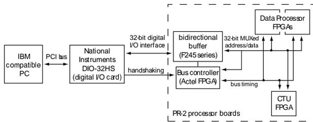
Figure 6: Test setup for data handling and control of the PR-2 processor. An IBM-compatible PC is interfaced to the PR-2's local address and data bus through a National Instruments Digital I/O board.
