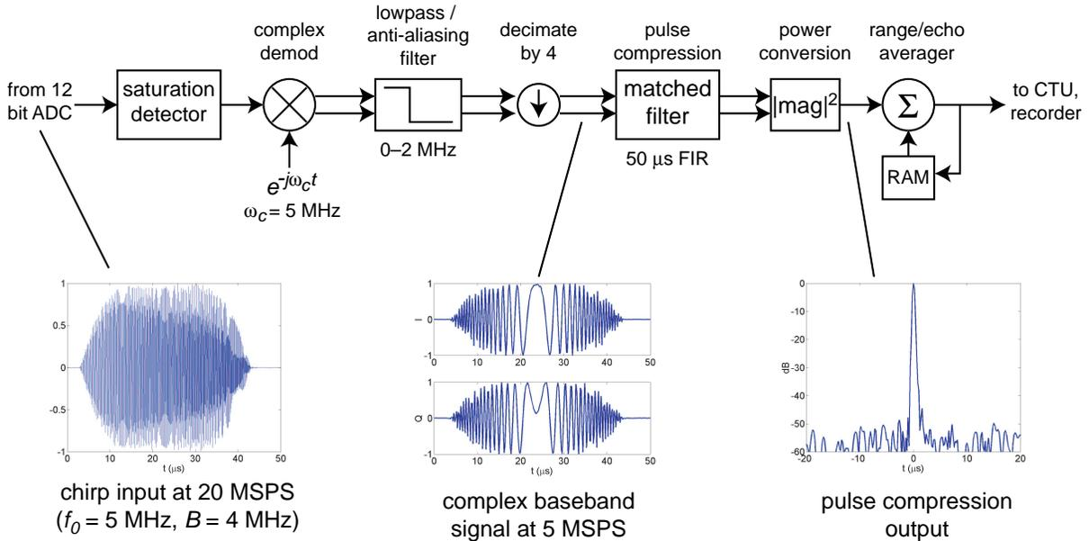
Figure 4: Functional block diagram of the digital data processor signal flow for the PR-2.
