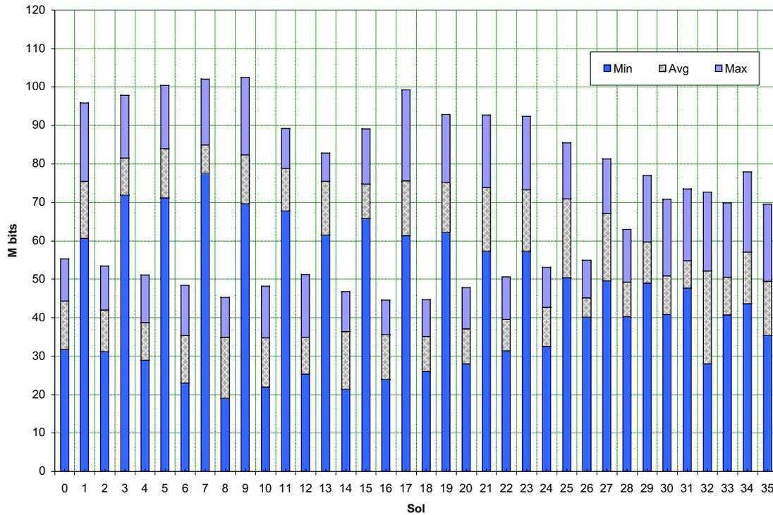
**Fig. 5-15. Data volume per sol in return link between MER and Odyssey for different rover orientations.**
