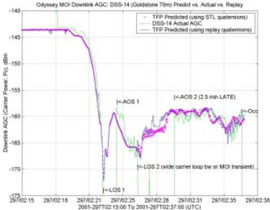
**Fig. 5-9. Post-MOI assessment: downlink  $P_{\text{carrier}}$  (AGC) predict versus actual versus replay.**
