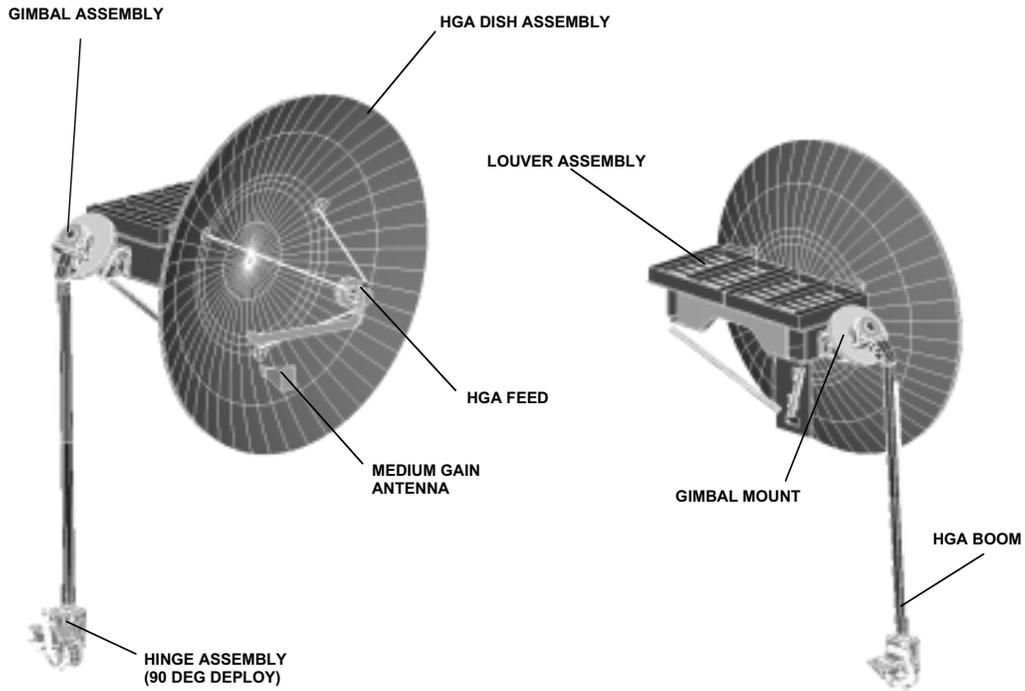
Fig. 3-5. Odyssey HGA, feed with MGA, and mount with gimbal.
