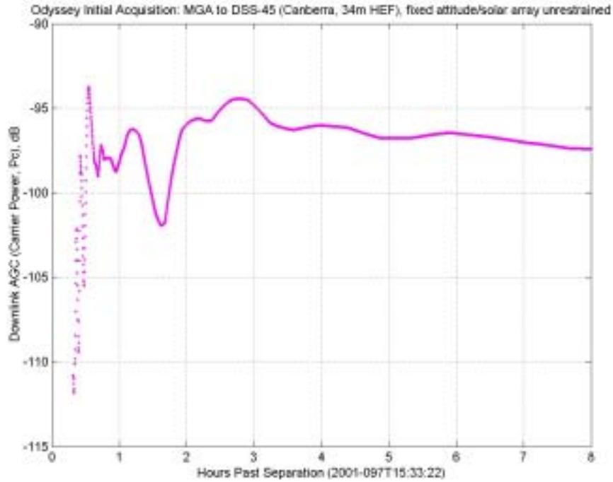
**Fig. 5-2. Downlink  $P_{\text{carrier}}$ , initial acquisition, fixed attitude with solar array unrestrained.**
