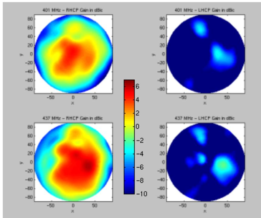
**Fig. 3-12. UHF antenna pattern as measured on the spacecraft.**
