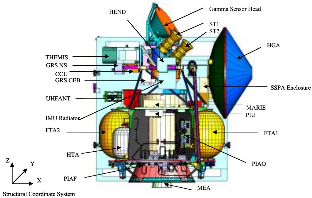
Fig. 3-2. Side view of the orbiter showing the stowed HGA and the SSPA enclosure.
