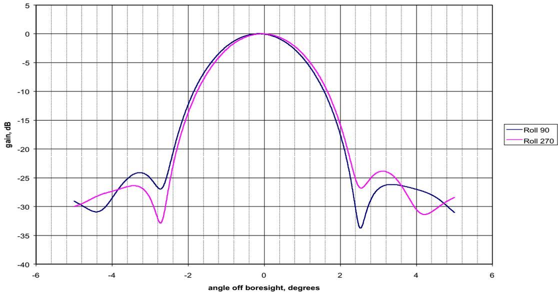
Fig. 3-6. HGA gain pattern, transmit.
