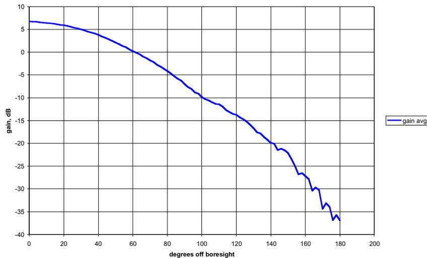
**Fig. 3-9. LGA receive gain pattern.**
