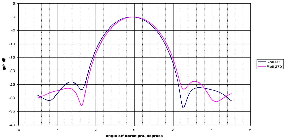
Fig. 3-7. HGA receive gain pattern.
