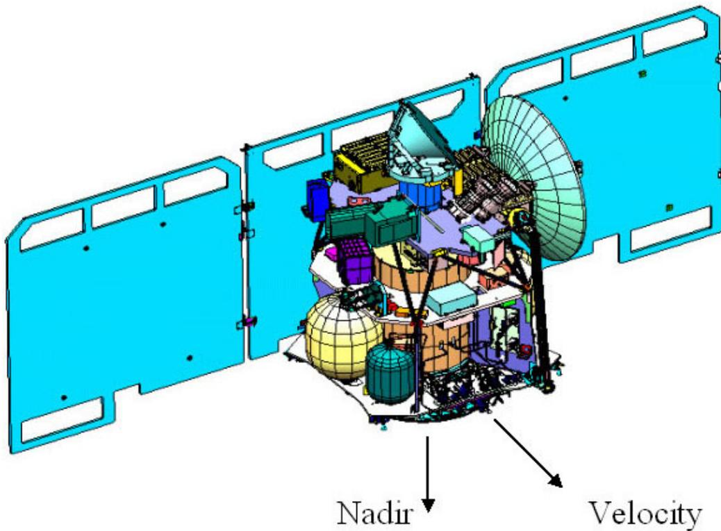
**Fig. 5-10. Odyssey configuration during aerobraking drag passes.**
