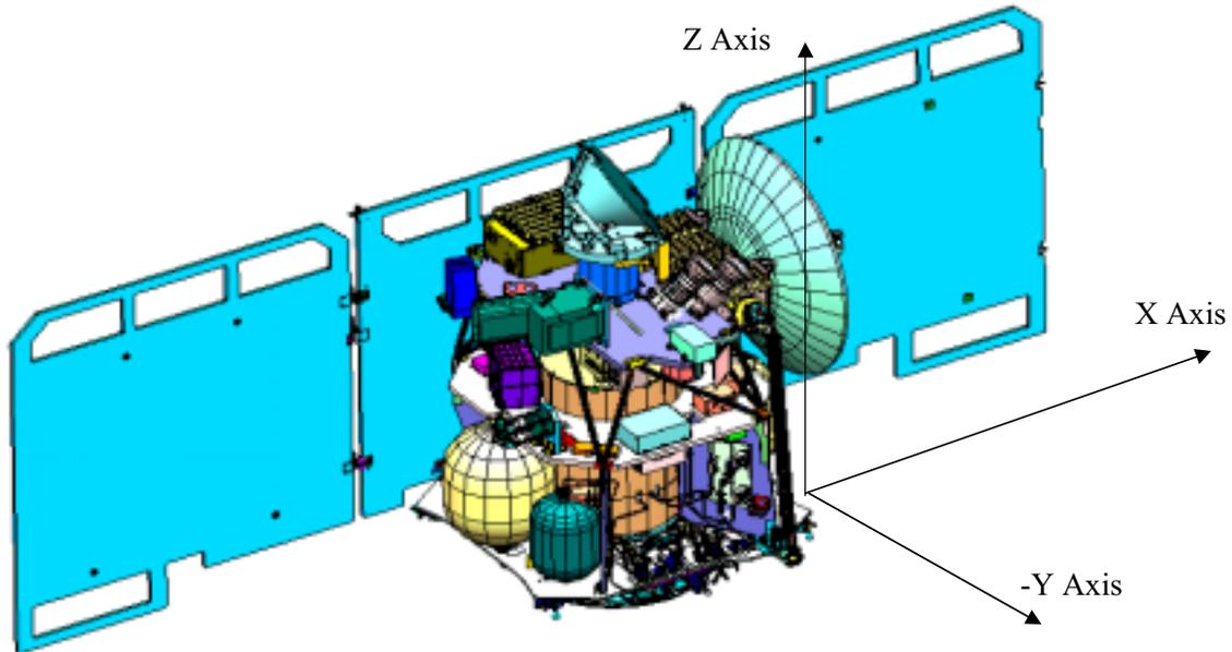
**Fig. 1-1. Overview of the orbiter configuration.**
