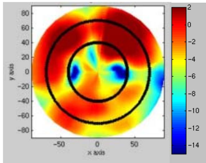
**Fig. 5-14. MER 401-MHz transmit antenna pattern, gain in dB.**
