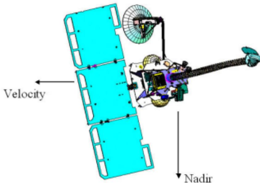
Fig. 5-13. Odyssey configuration during the relay phase.
