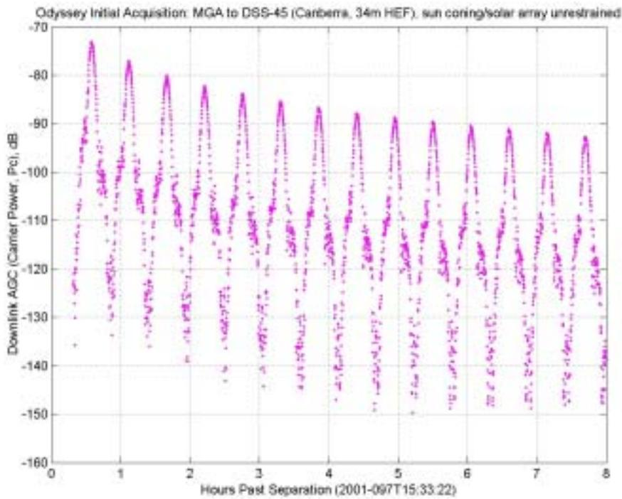
**Fig. 5-3. Downlink  $P_{\text{carrier}}$ , initial acquisition, Sun coning/solar array unrestrained.**
