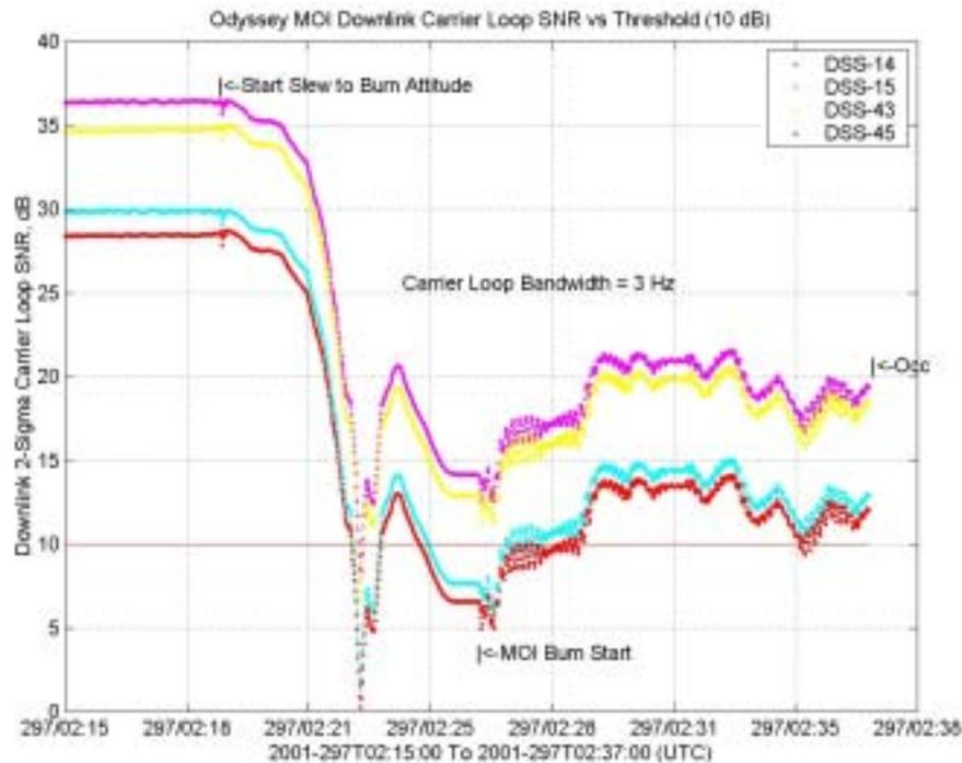
**Fig. 5-8. Predicted downlink carrier loop SNR (3-Hz bandwidth).**
