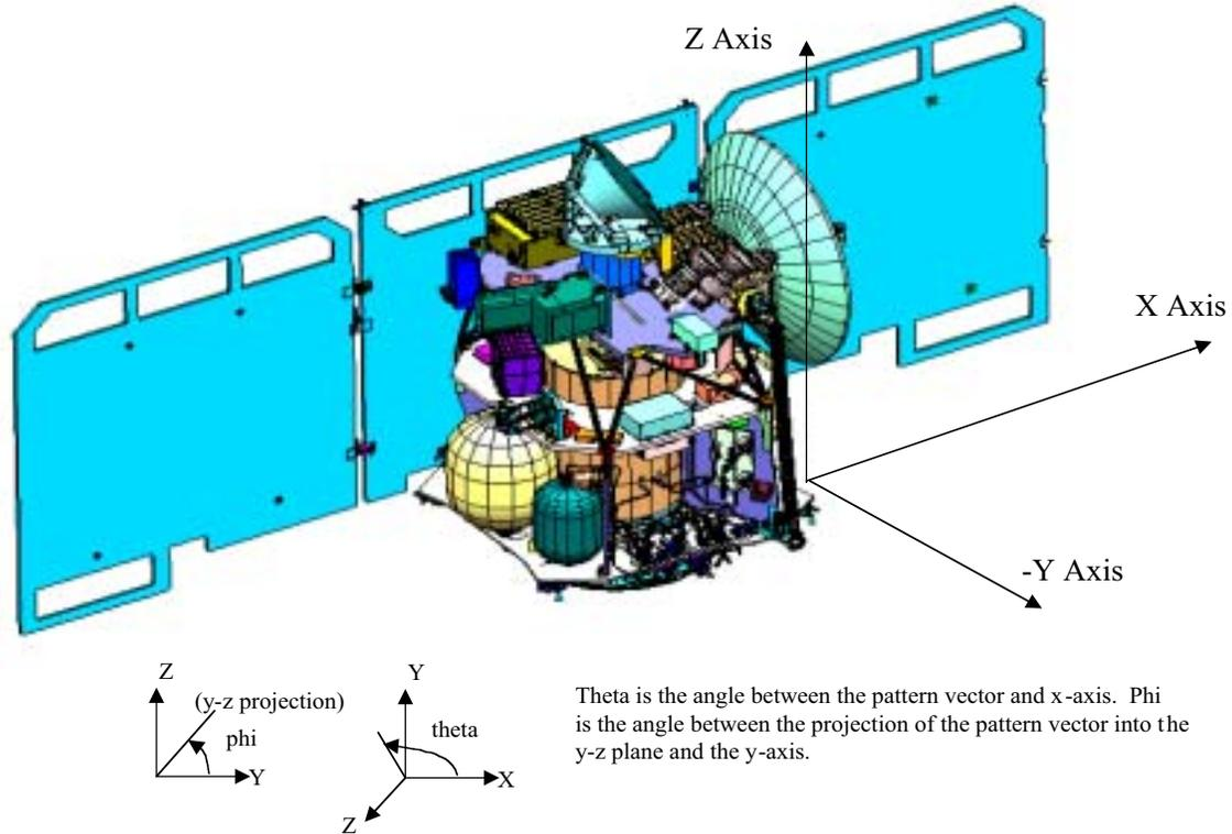
**Fig. 5-6. Cone ( $\theta$ ) and clock ( $\phi$ ) with respect to the spacecraft body frame.**
