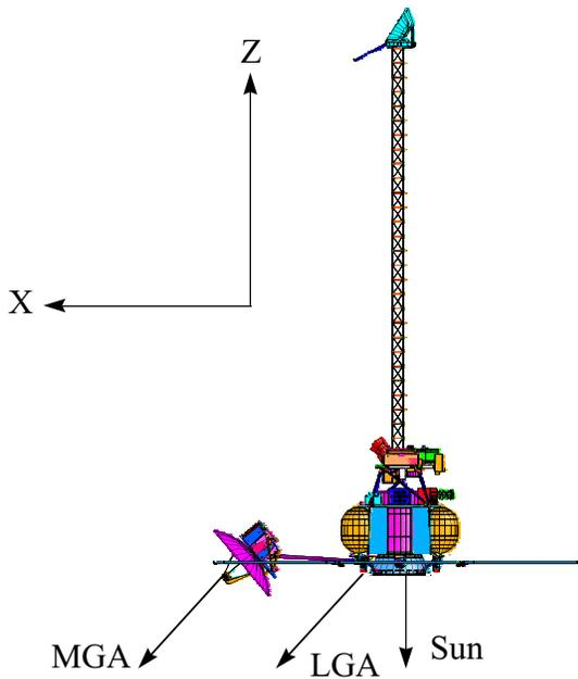
Fig. 1-8. Safe mode attitude during the science and relay phase.
