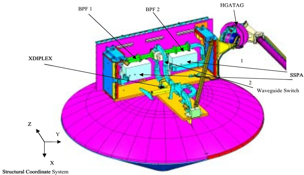
Fig. 3-3. Layout of the orbiter X-band telecom components in the SSPA enclosure.
