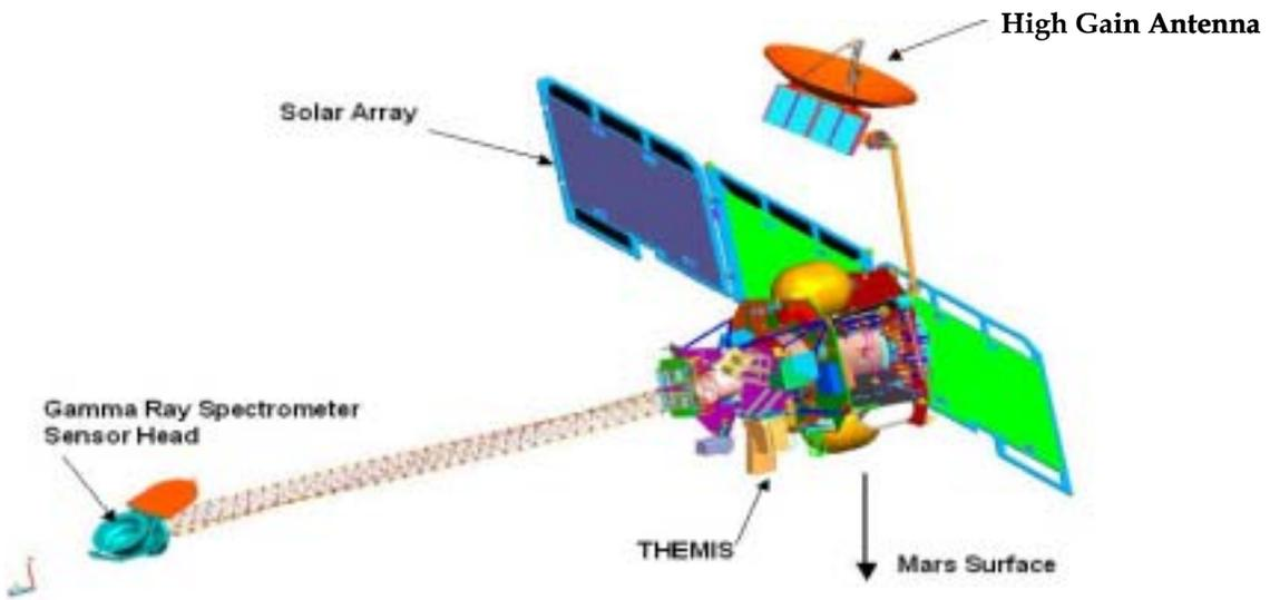
Fig. 5-12. Odyssey mapping configuration during the science phase.
