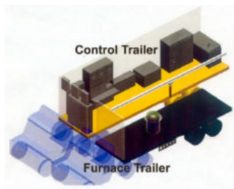
**Figure 5. Conceptual Modular, Transportable Melt-Dilute System**
