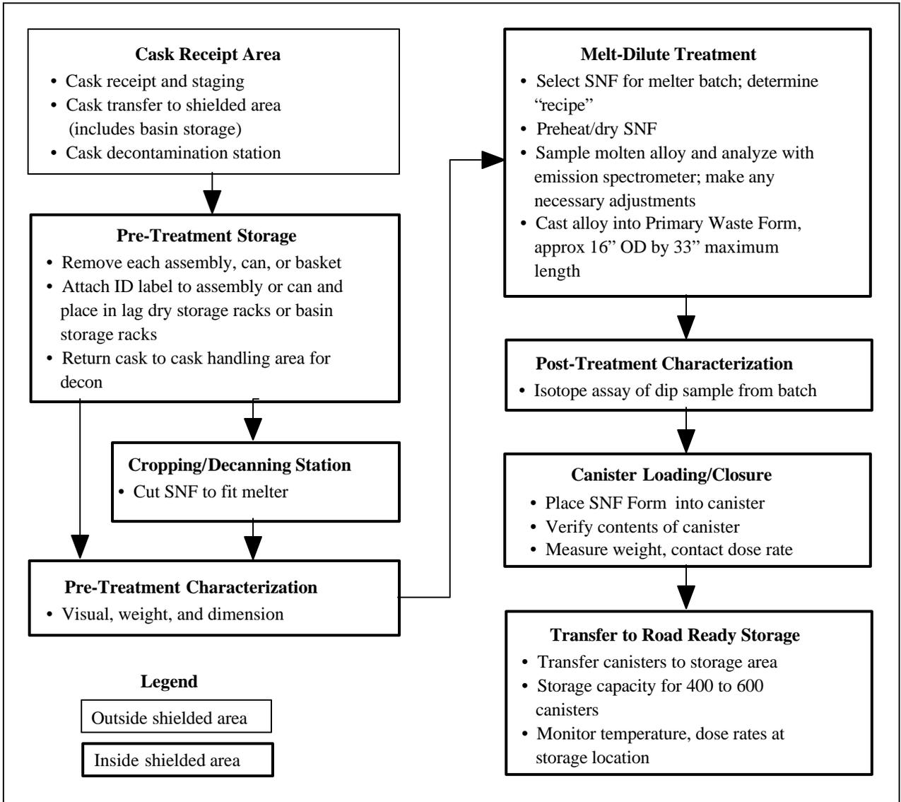
Figure 1. Process Steps in TSF for Melt-Dilute Technology
