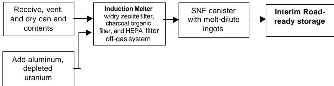
**Figure 4. Flow diagram for Metallurgical Mounts using the Melt-Dilute Treatment technology**
