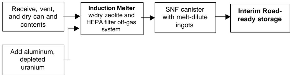
**Figure 2. Flow diagram for U233-CEUSP using the Melt-Dilute Treatment Technology**
