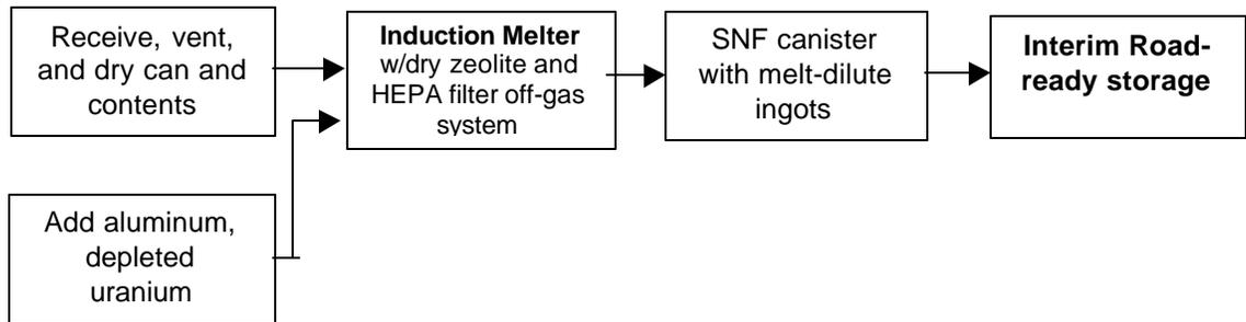
**Figure 3. Flow diagram for Pu-contaminated HEU and DU/Off-spec HEU using the Melt-Dilute Treatment Technology**
