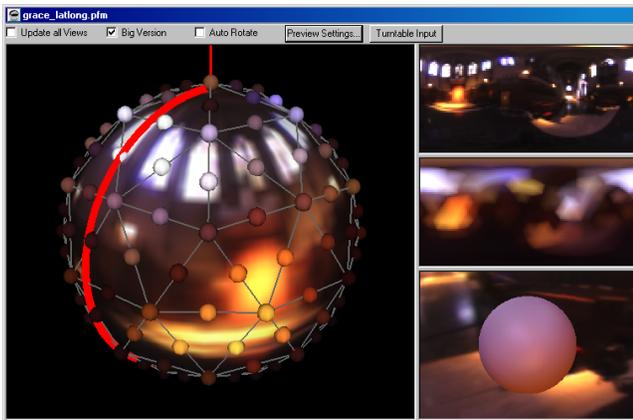
Figure 9: **The Lighting Control Program**, showing the longitude/latitude image of incident illumination (upper right), the triangular resampling of this illumination to the light stage’s lights (middle right), the light colors visualized upon the sphere of illumination (left), and a simulated sphere illuminated by the stage and composited onto the background (lower right).
