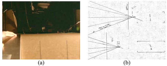
Figure 10: **Measuring Nodal Point Location and Field of View** (a) The nodal point and field of view of each camera were measured by setting the camera on a horizontal piece of cardboard (a) and drawing converging lines on the cardboard corresponding to vertical lines in the camera’s field of view. (b) The field of view was measured as the angle between the leftmost and rightmost lines; the nodal point, with respect to the front of the lens, was measured as the convergence of the lines.
