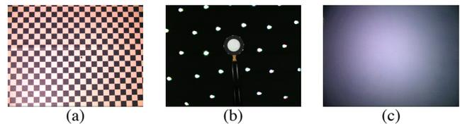
Figure 11: **Geometric and Photometric Calibration** (a) The calibration grid placed in the light stage to align the infrared camera image to the color camera image (b) A white reflectance standard imaged in an even sphere of illumination, used to determine the mapping between light colors and camera colors (c) A white card placed in the light stage illuminated by all of the lights to calibrate the intensity falloff characteristics.
